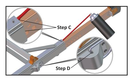
**Step C:** Extend the Ratchet<sup>™</sup> Leveler. Using the **Dry Lubricant** generously apply to the top, bottom and sides of the internal leg leveler (as shown in the illustration), clean off any excess lubricant.
