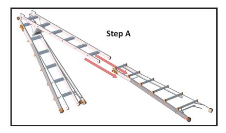
**Step A:** Remove the outer assembly from the inner assembly.
